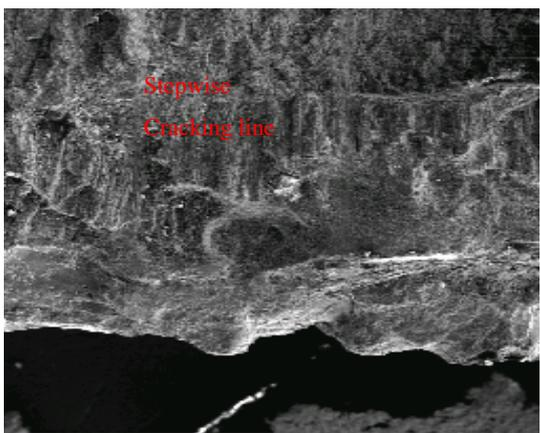
Fig. 10 morphology of tensile fractured surface
