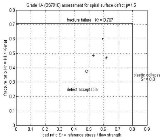
Fig.4 FAD at p=4.5 MPa
