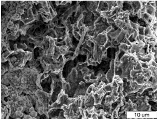
Fig.8 fractograph near internal surface
