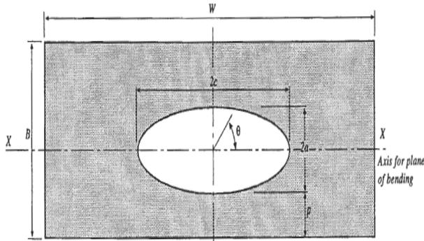
Fig.2 Axial embedded defect
