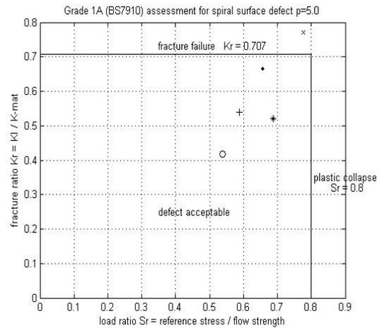
Fig.5 FAD at p=5.0 MPa
