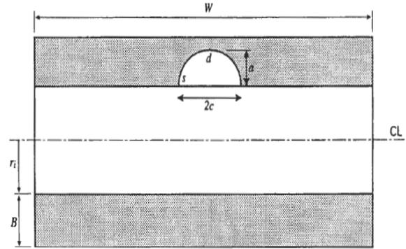
Fig.1 Axial defect on internal surface
