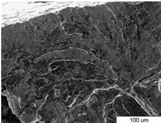
Fig. 9 morphology of cleavage fracture
