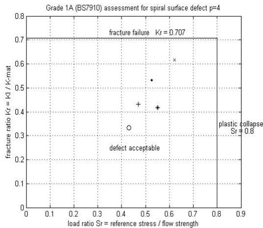
Fig.3 FAD at p=4 MPa
